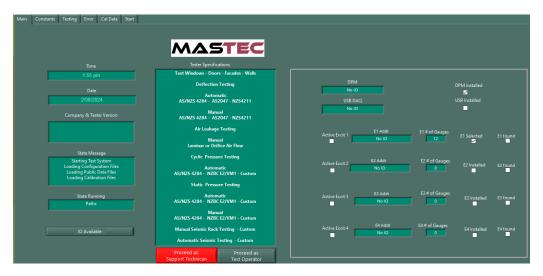
The Testing TAB's FP is the display where the Operator and Commissioner can drive all the systems functions and options. (Commissioning, Checking, Calibrating, Testing)
